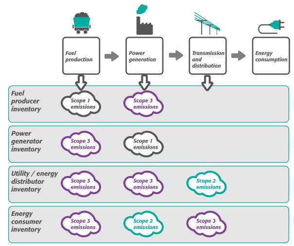
Figure B.1 Accounting for electricity emissions throughout the supply system
