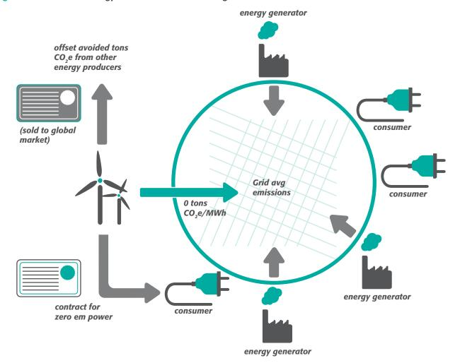
Figure 8.1 Offsets and energy attribute certificates on a grid
