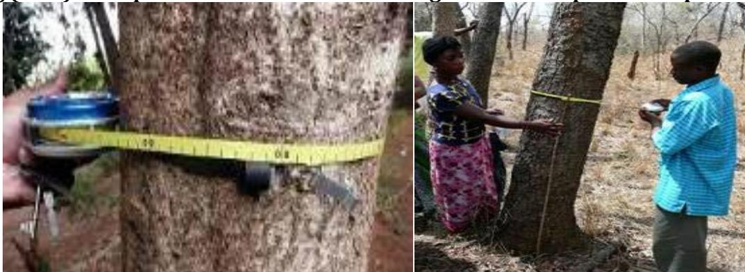
Above Dbh Measurement with Diameter Tape and below with Caliper
