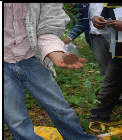
Figure 2 using a sharp field knife, any excess soil over the core should be removed to ensure a volumetric soil sample
