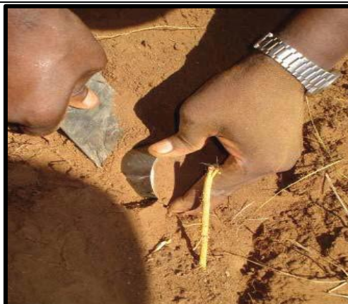
Figure 3: The core with soil sample is extracted carefully from the wall of the pit, using a trowel or a knife if necessary
