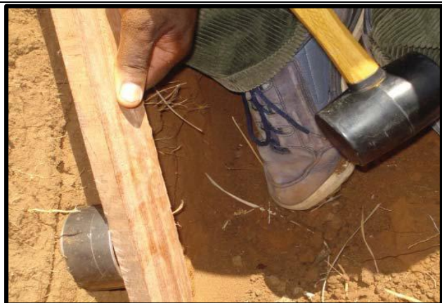
Figure 2: The sampling cylinder is pushed into the wall with a plastic hammer. When hammering, it helps to cover the cylinder with a wooden plank
