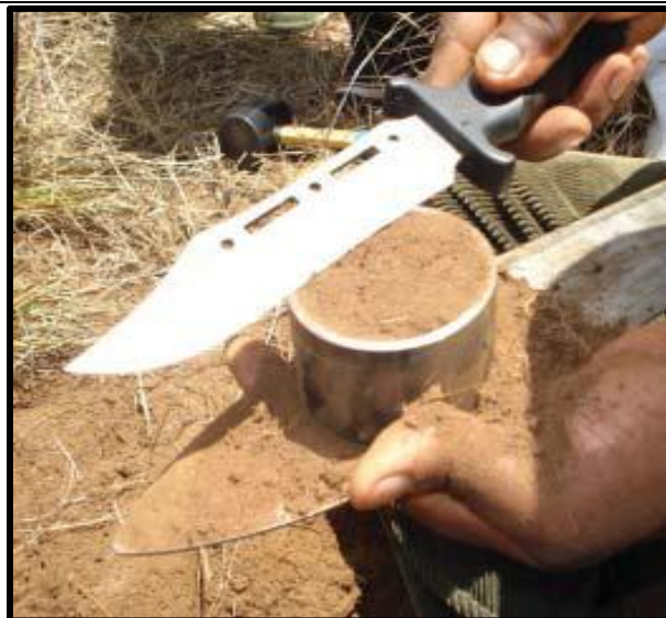
Figure 2 using a sharp field knife, any excess soil over the core should be removed to ensure a volumetric soil sample
