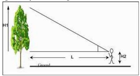
Fig (4.13) Height measurement using a hypsometer
