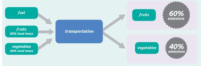
In figure 9.3, the amount of fruits and vegetables the truck transports are limited by the mass of the products. However, if the fruits and vegetables are transported by rail and the limiting factor is the volume of products, the most appropriate allocation factor would be volume.
