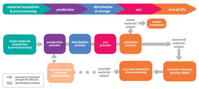
Figure [9.5] Example process map illustrating the closed loop approximation method
