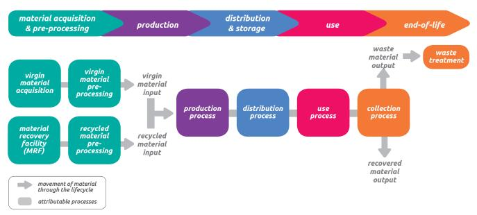
Figure [9.6] Example process map illustrating the recycled content method
