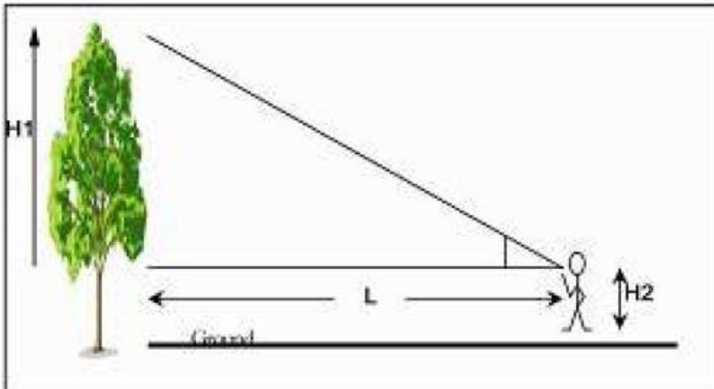
**Fig (4.13) Height measurement using a hypsometer**
